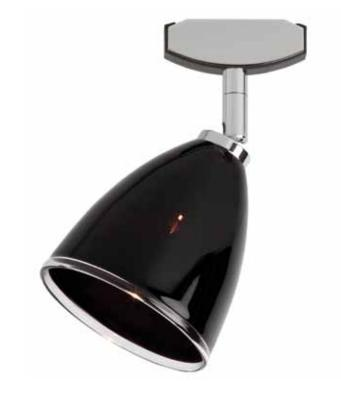
**Spot Unica Mini** for Magnetline. Made of hand-blown glass. Each glass is unique and signed by the glass artist. Height of glass: 110 mm Diameter of glass: Ø 100 mm Energy efficiency category: B - D Socket: GY6,35 max. 12 V/50 W
